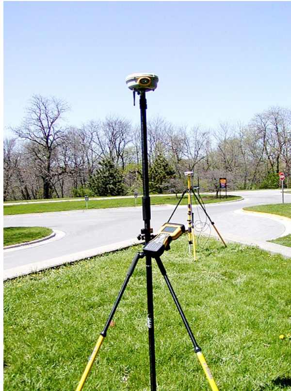
FIGURE 11. Two GNSS receivers mounted on rods stabilized by tripods. From Flickr user “Manop”: https://commons.wikimedia.org/wiki/File:Station_GPS_receiver.jpg .
