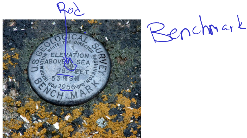
FIGURE 2. Survey benchmark in the USA. Their locations are measured and recorded very accurately, and can be accessed in local and national databases.
