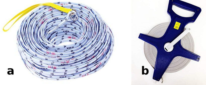
FIGURE 3. (a) Surveyor's "rope". (b) open-reel measuring tape, also often used in surveying.
