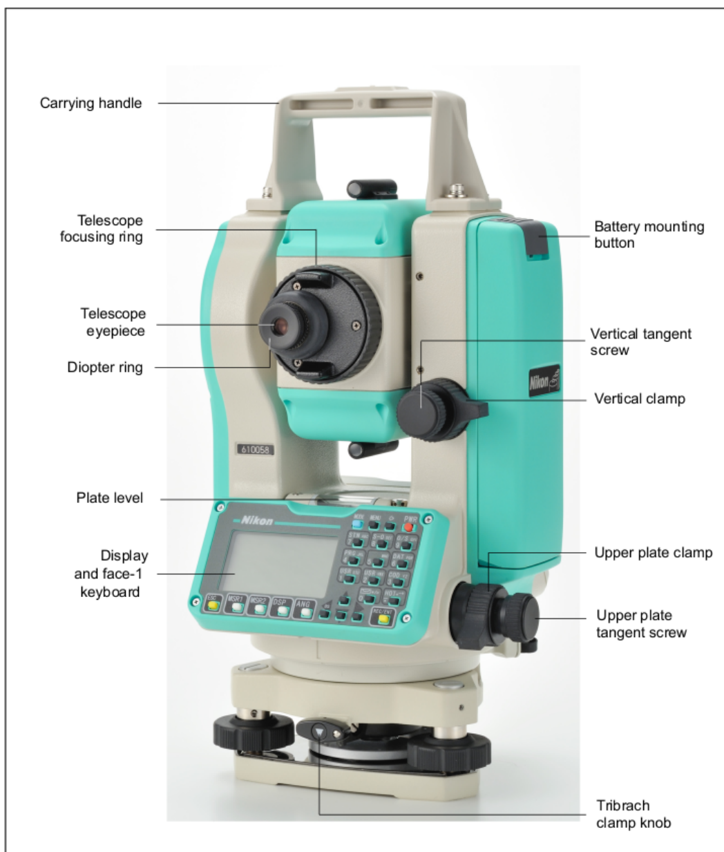
FIGURE 13. Nikon DTM-322, Face 1. From Nikon user's manual.
