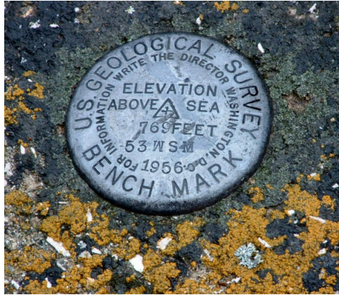
FIGURE 2. Survey benchmark in the USA. Their locations are measured and recorded very accurately, and can be accessed in local and national databases.
